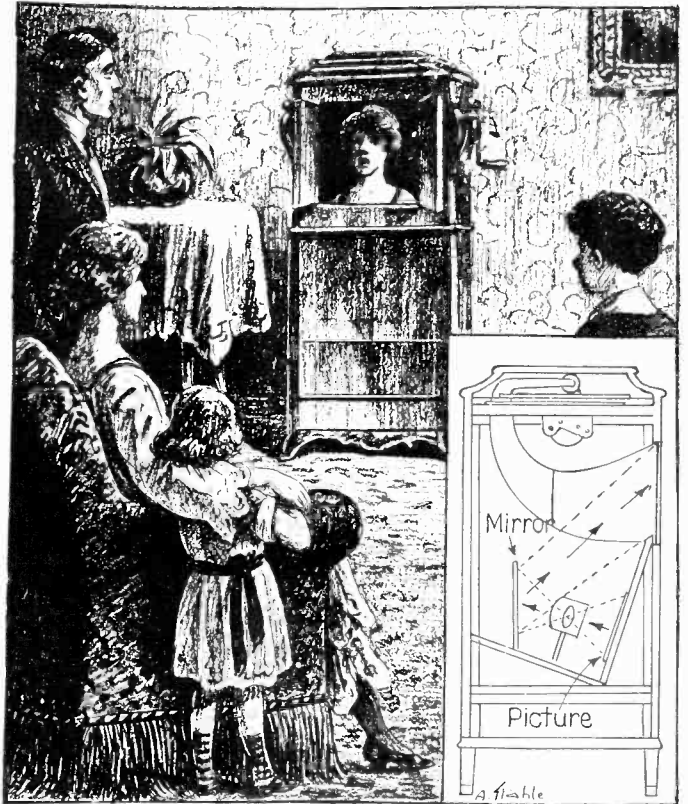
The inventor of this device, Robert A. Rummel, makes it possible to see the singer at the same time her record is heard on the phonograph. The device consists of a reflecting projector placed in the base of the musical instrument.
